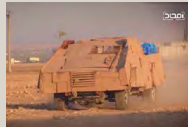
An up-armored SVBIED based on a pick-up truck used against a Syrian loyalist position near Abu Dali/Mushayrifa in eastern Hama on Oct. 8, 2017.
