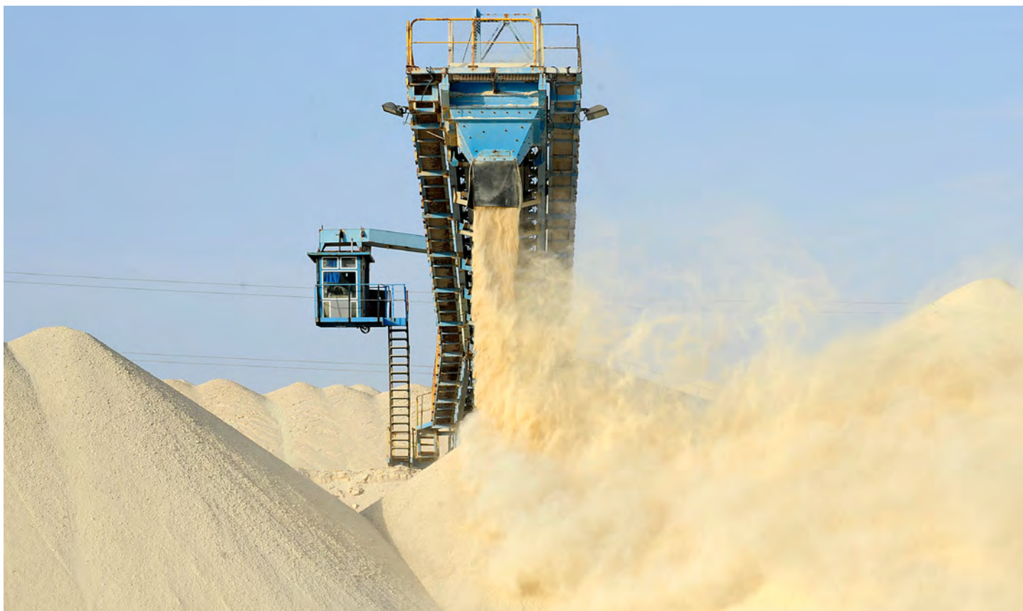
Photo above: Untreated phosphate being dropped off on a mountain at the end of a conveyor belt at the OCP's Marca factory, near Laayoune, Western Sahara. Photo by FADEL SENNA/AFP via Getty Images .
